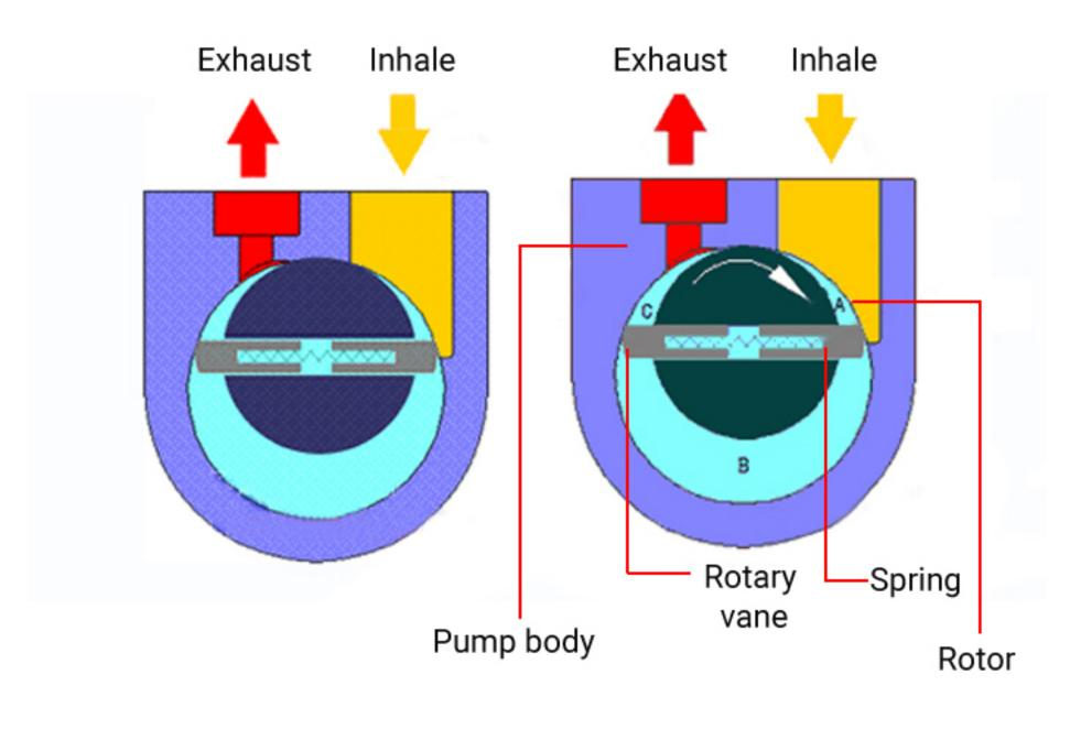
Rotary vane pump is mainly composed of pump body, rotor, rotary vane, end cover, spring, etc. Installing a rotor in rotary vane pump cavity, the outer circumference of the rotor is tangent to the inner surface of the pump chamber and the rotor slot inner
